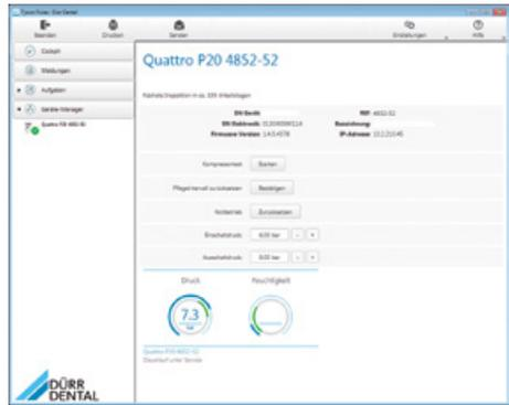
With the aid of Tyscor Pulse the pressure of the compressor can be adjusted as required.
