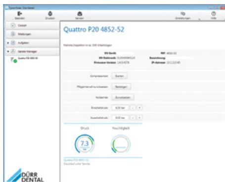
The compressor can be manually started with the aid of Tyscor Pulse.
