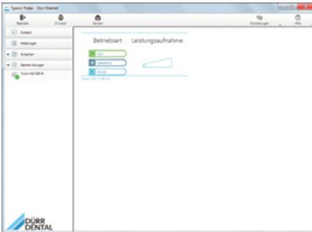
The suction unit can be used in various operating modes. Depending on the installation situation and power requirements, one of the following operating modes can be selected: Eco, Balanced or Boost. On delivery, the suction machine is set to Balanced.
