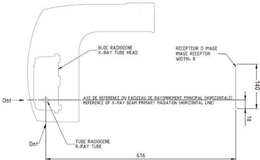
**Table 7 Technical Specifications of the X-ray tube Assembly**
