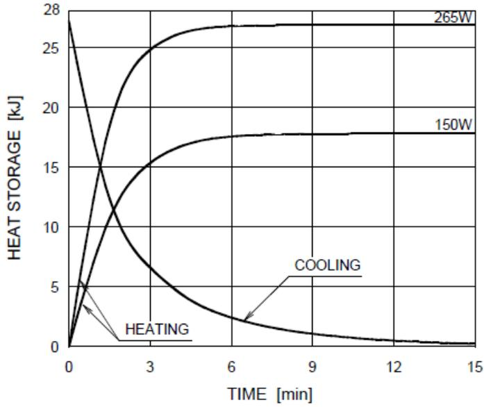
**Figure 4 Heating and Cooling Curves of the X-ray Tube OX/120-0307**
