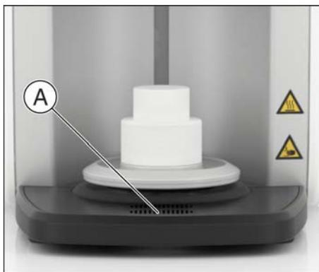
1. As soon as the processes have completed, use the fireproof tray of the CEREC SpeedFire to support your restoration while it is still hot and cool it to room temperature. Use tweezers to help you unload the furnace.
