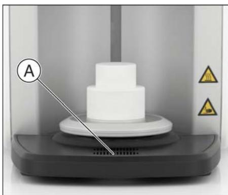
5. As the restoration is still very hot in this phase, only unload the furnace using metallic or ceramic tweezers and do not touch the restoration directly. Plastic tweezers are not suitable for removing restorations. Place the restoration on the fire-proof tray (A) for further cooling – avoid the draft.
