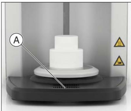
5. As the restoration is still very hot in this phase, only unload the furnace using metallic or ceramic tweezers. Plastic tweezers are not suitable for removing restorations. Place the restoration on the fireproof tray (A) for further cooling (see “Fireproof tray with integrated fan [ → 48]”).
