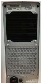
Under no circumstances may the ventilation slots on the rear of the unit be covered, since otherwise the air circulation will be obstructed. This can cause the unit to overheat.
