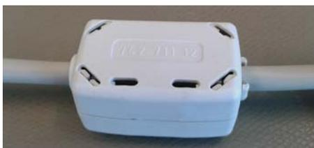
1. Place the network cable into the open ferrite core.
