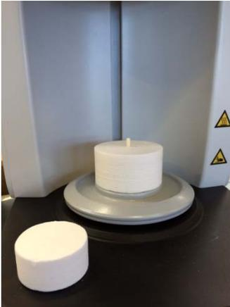
2. Start by placing the bottom door insulation on the positioning pin.
