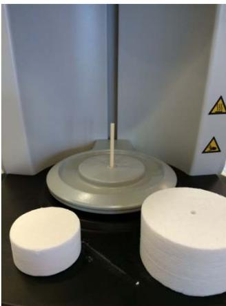
1. Insert the positioning pin into the hole of the furnace door.
