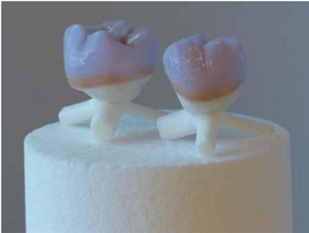
For multi-jobs, a maximum of two individual tooth restorations can be positioned together in the furnace.
