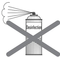
Do not spray liquids such as disinfectants into the ventilation slots. This may lead to malfunctions. Use wipe disinfection only in the vicinity of the ventilation slots.
