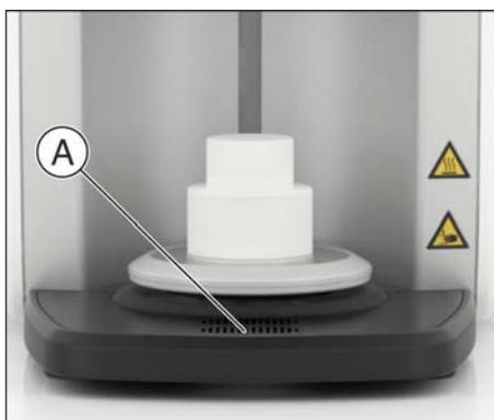
3. As the restoration is still very hot in this phase, only unload the furnace using metallic or ceramic tweezers. Plastic tweezers are not suitable for removing restorations. Place the restoration on the fireproof tray (A) for further cooling (see "Fireproof tray with integrated fan [ → 48]").
