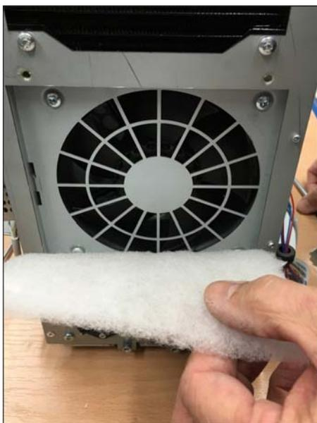
3. Remove the contaminated filter fleece and insert the new filter fleece.
