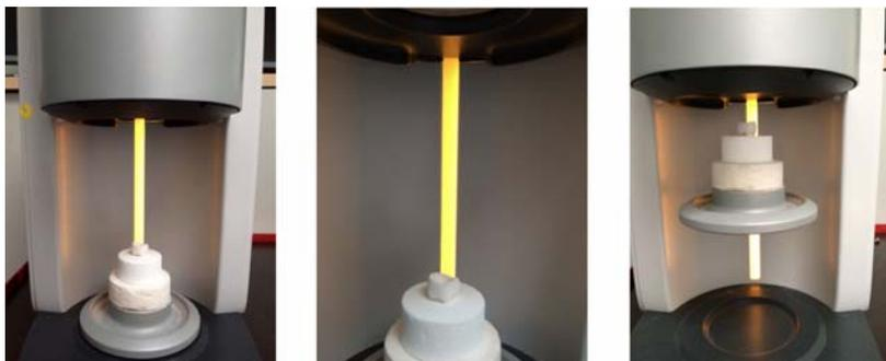
1. Place the restoration with the occlusal surface facing downward on the top door insulation. The restoration must not protrude from the insulation surface, as this might cause a collision with the furnace chamber insulation.
