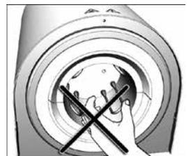
Do not touch the thermocouple and the heating element in the sintering chamber. Avoid contact with the skin (grease contamination), as the parts may be prematurely damaged.
