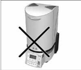
For safety reasons, the furnace must not be operated without the cooling tray.
