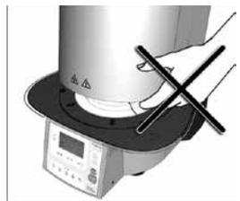
The furnace head is equipped with an electric drive and can be operated by means of the electronic controls. Never open the furnace head by hand, since this will damage the transmission.
