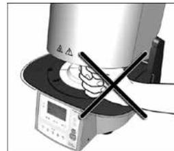
Never reach under the furnace head with the hand or other parts of the body during operation, since there is a risk of crushing and a burn hazard.
