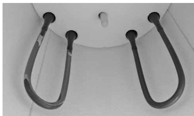
Large parts of the protective layer on the left heating element have chipped off. The heating element on the right side is in a sound, stable condition and shows an intact oxide / protective layer. The cleaning program must be repeated until the surface is free from contamination and appears glassy.
