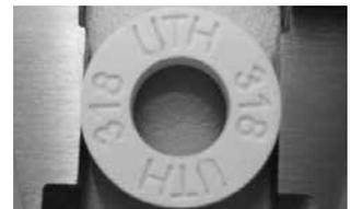
6. Find the measured diameter in the conversion table and read off the corresponding temperature. Only if the deviation is more than 5 °C must the furnace be readjusted.
