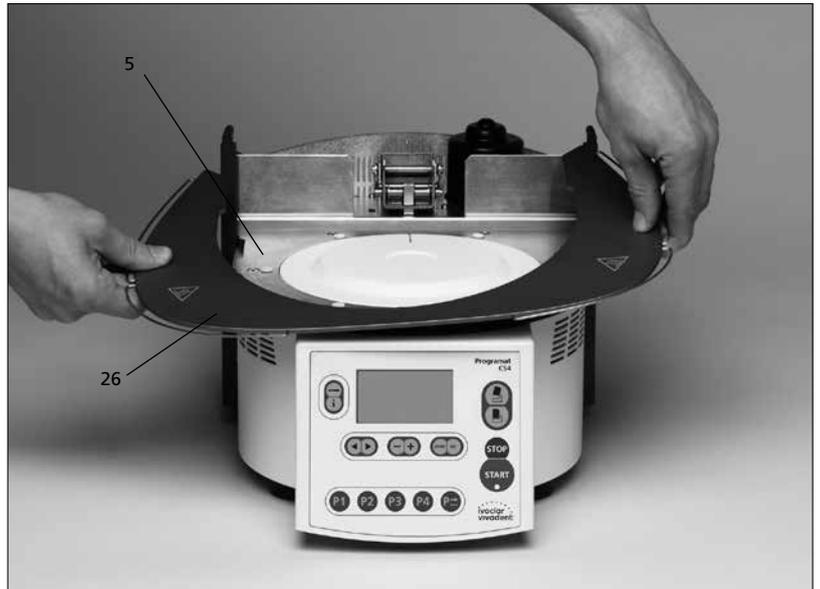
Secure the cooling tray (26) with the two screws (27) including the silicone washers (28).
