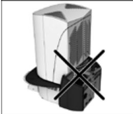
The furnace must not be connected to the power supply without the rear cover in place.
