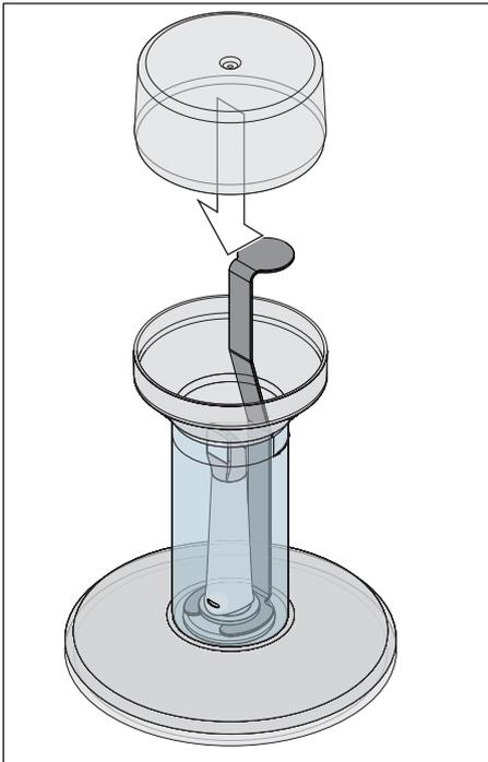
10. Place the cover on the container and leave the mirror sleeve in the disinfectant for at least 12 minutes (CIDEX<sup>®</sup> OPA). The mirror sleeve will not be damaged if it remains in the disinfectant for longer than the required time, but removing it shortly after the required time is recommended.
