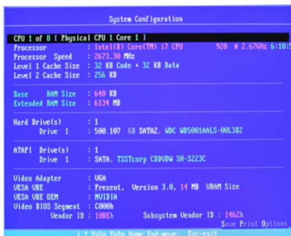
1. Using the information in the system configuration, check whether the system corresponds to the default settings. You can scroll up and down using the arrow keys.
