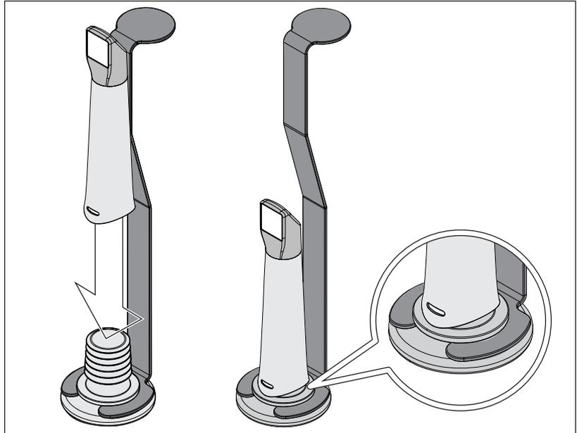
7. Press the mirror sleeve onto the plug while holding the metal bracket firmly in place in order to ensure that no particle contamination or fluids penetrate the inside of the mirror sleeve.
