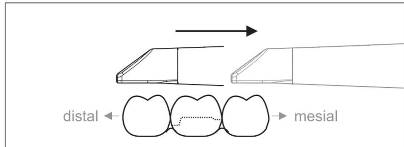
**Important:** Ensure that the distance between the coated sapphire glass of the CEREC Omnicam and the scanned surface is observed. The distance must be between 0- 15 mm (ideally: 5 mm). The camera does not rest on the teeth or the gums. If the distance is too great, no data will be obtained.
