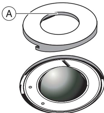
1. Rotate the cover ring counterclockwise and remove it.
