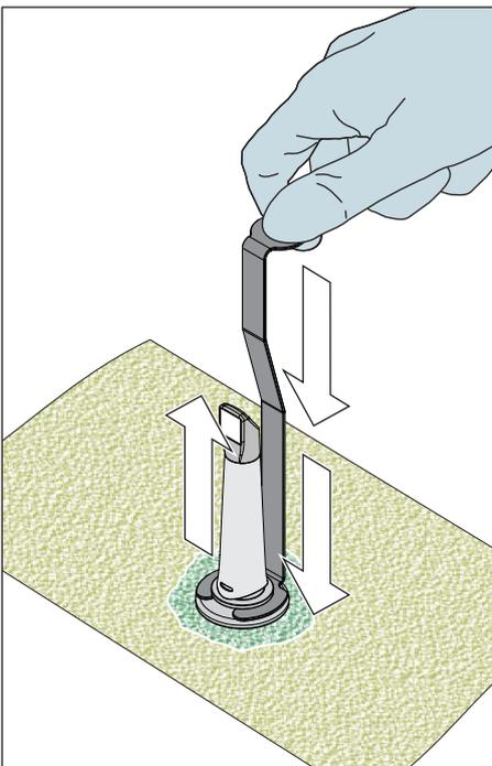
13. Remove the bracket from the mirror sleeve carefully and slowly by pushing the bracket downwards. Ensure that the mirror sleeve is pointing upwards so that no fluids are able to penetrate into the interior of the mirror sleeve.
