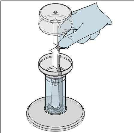
11. Remove the cover and take the bracket with the mirror sleeve out of the container.
