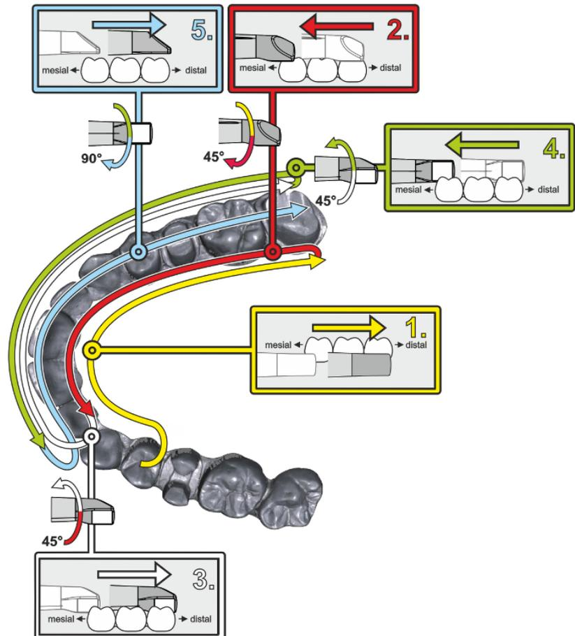
1. Start by placing the device on the occlusal surface of a premolar, that has already been scanned, and guide the camera palatally (orally) at a mesial tilt of up to 90° across the lingual surface of the front teeth in a distal direction towards the terminal tooth.
