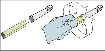
17. Dry the entire outer surface of the mirror sleeve as well as the inner section using a soft lint-free cloth. Ensure that no fluid is able to penetrate the inside of the mirror sleeve.
