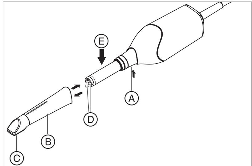
1. Press the mirror sleeve (**B**) against the camera body.
