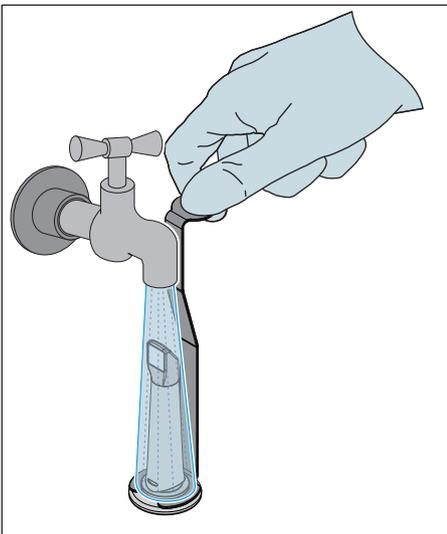
12. Carefully rinse the mirror sleeve with tap water for at least 30 seconds while holding it with the bracket.
