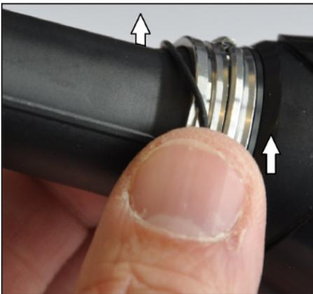
2. Starting from this point, carefully use your thumb and index finger to push the O-ring into the groove (in a similar way to pushing it out but without any force).
