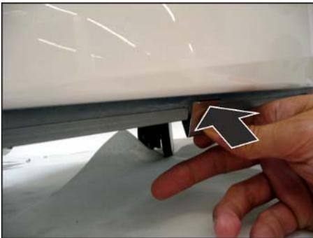
5. Open up the lengthways cover by pushing the lateral spring plate.
