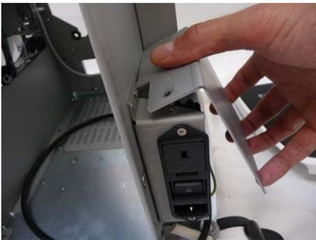
8. Insert the plate cover at the top and tilt it downwards.
