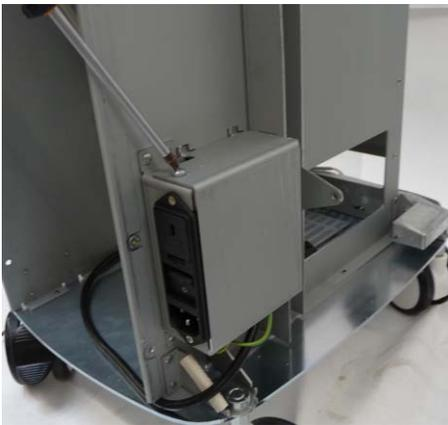
9. Screw on the screw of the plate cover.
