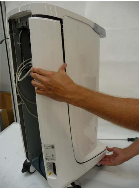
4. Remove the left cover by pulling it out downwards slightly and then to the rear.
