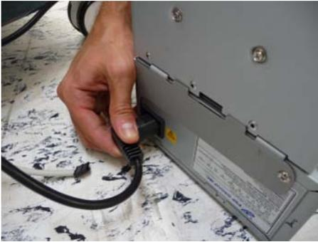
10. Detach the connector of the power supply from the rear side of the power supply unit.
