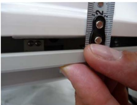
3. The optimum switching point is reached when the clearance of an engaged but not actuated footswitch is approximately 6–7 mm.
