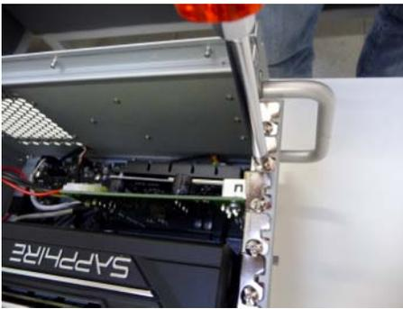
2. Remove the screw from the PCI slot plate and pull the WLAN card up and out of the PC.
