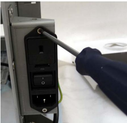
5. Unscrew the 2 screws (A) and remove the power input.
