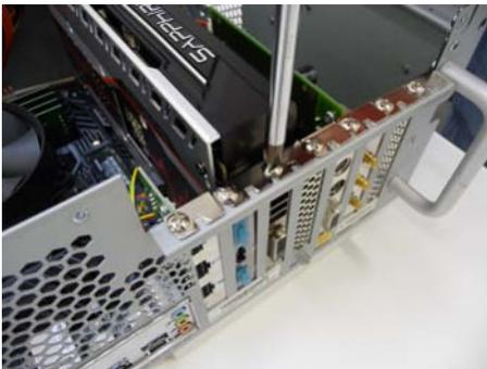
5. Remove the 2 screws of the PCI slot plate.
