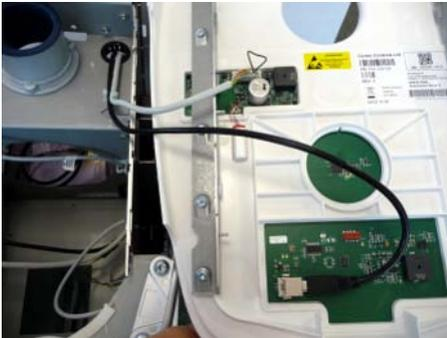
2. Attach the USB connector and the connector of cable L1 and route the cable as shown.
