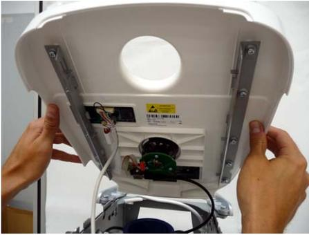
5. Raise the complete control unit upwards slightly and carefully.
