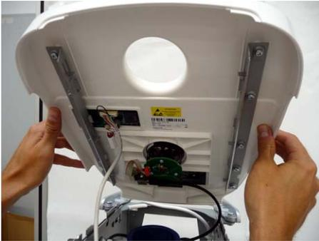
1. Hold the control unit raised up slightly over the acquisition unit.
