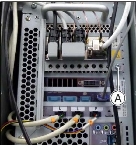
5. Unscrew the locking plate mini DIN connector (1 screw **A**).
