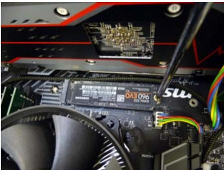
5. Screw the SSD module down tightly with the fastening screw.
