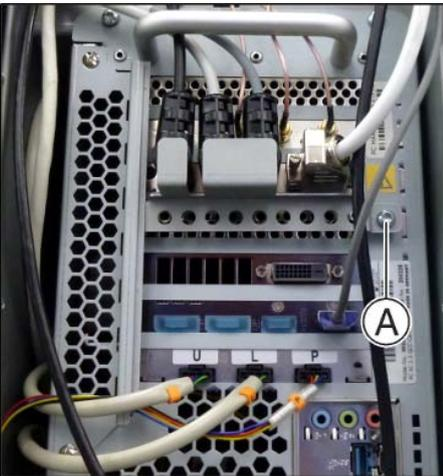
8. Re-tighten the locking plate mini DIN connector with 1 screw (A).
