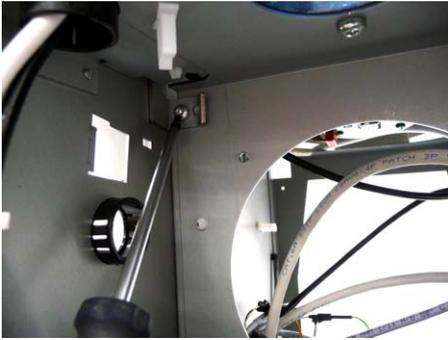
4. Push the left locking plate forwards up to the stop and then screw it back on again with the screw. Perhaps help things along by simultaneously pressing the control unit downwards slightly on the relevant side.
