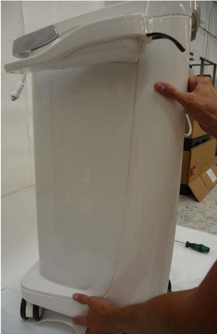
4. Remove the right cover by pulling it out downwards slightly and then to the rear.
