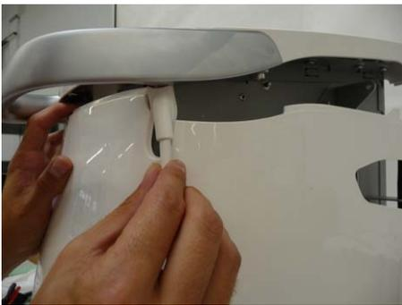
4. Paying attention to the scanner cable, press the front cover downwards slightly and pull it forwards and out.
