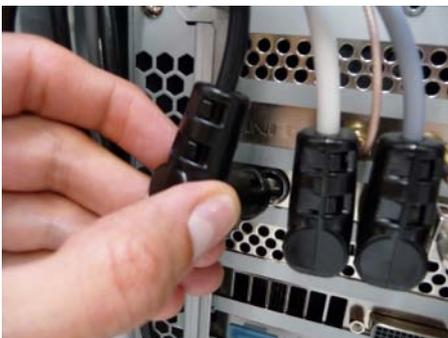
5. Route the cable (L4) behind the handle and insert the mini DIN connector into the socket (X101) of the supply board.
