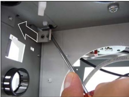
3. Use the blade screwdriver as a lever and push the locking plate back up to the stop.
