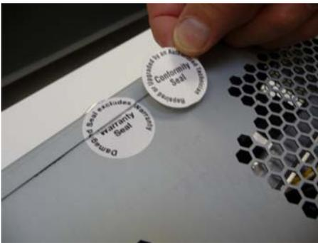
4. Attach the technician's conformity seal provided as shown.
