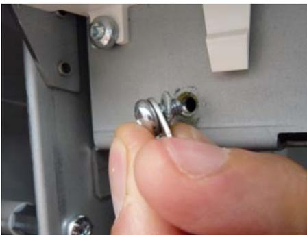
4. Insert the eyelet of the ground cable (L14) as shown between the screw head and tooth washer. Fasten the ground cable using the screw.
