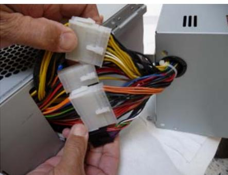
4. Disconnect the 4 plug connections and dispose of the defective power supply unit.
