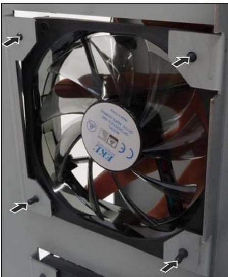
1. Pull the fan sleeve with fan inwards and out.
