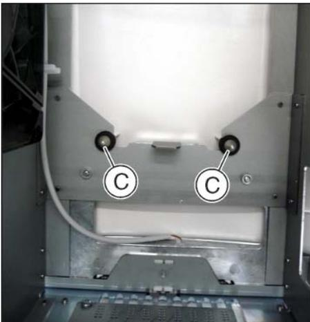
3. Press the 2 Pilsz connectors (C) from behind out of the grommets.
