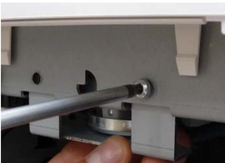
3. Screw the monitor brake on again as shown with the 2 screws.
