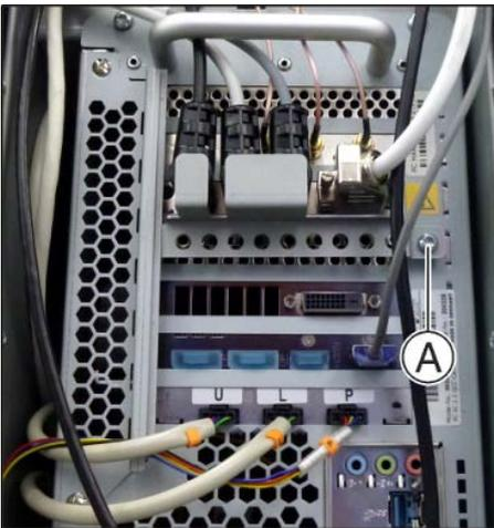
7. Re-tighten the locking plate mini DIN connector with 1 screw (A).
