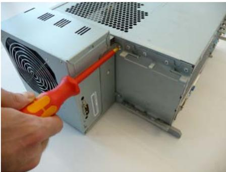
7. Screw the power supply unit on tight with the 2 fastening screws.
