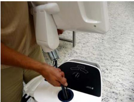
1. Guide the 4 monitor cables through the opening and insert the monitor.
