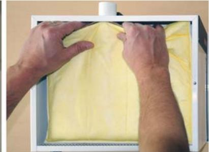
3. Remove the filter bag from the nozzle and put a new filter bag on.
