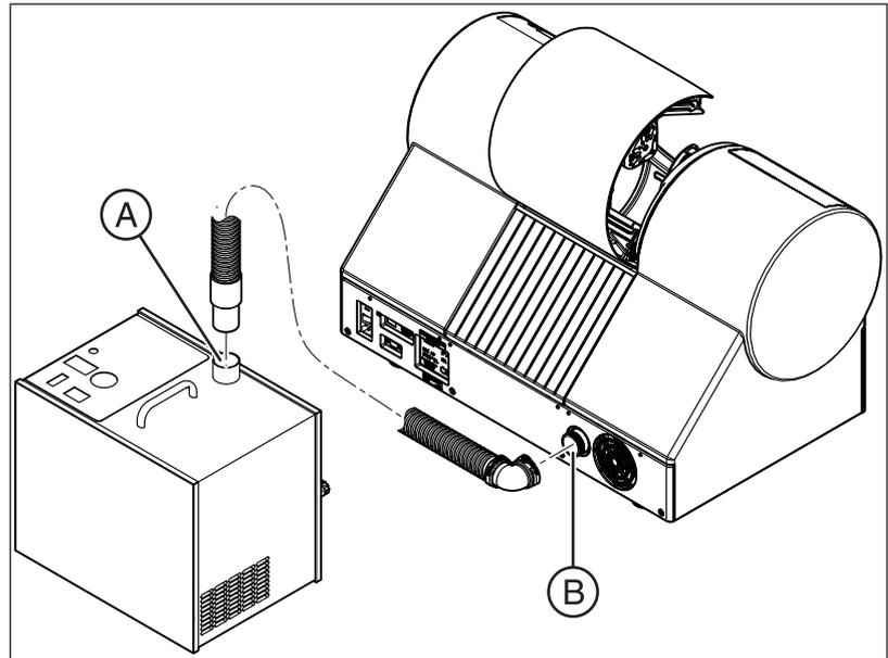
1. Connect one end of the suction tube to the available connection point on the suction device (A).
