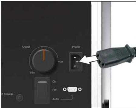
1. Insert the power cable into the relevant socket on the suction system.
