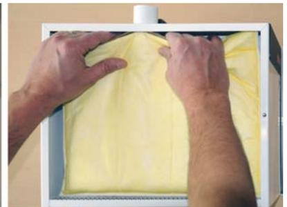
3. Remove the filter bag from the nozzle.
