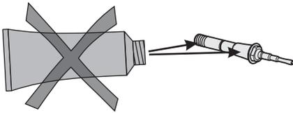
7. **NOTE! Do not grease the instrument!** Insert the new instrument into the motor mount by hand. Tighten the corresponding chuck with the torque wrench until a clicking sound can be heard.
