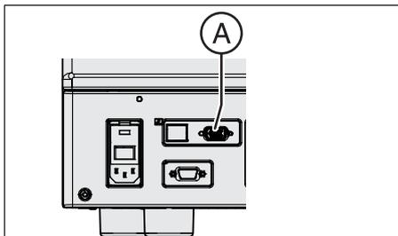
1. Plug the 15-pole connector into the socket (A) of the processing machine.
