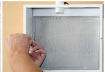
4. Then release and remove the two Phillips screws on the perforated sheet on the inside of the suction system.
