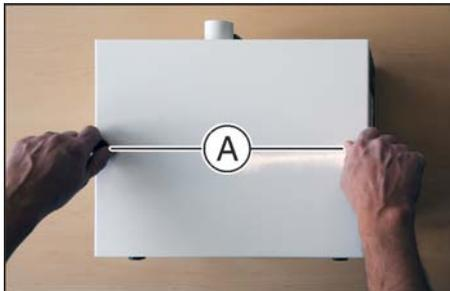
1. Loosen the two knurled nuts (A) on the maintenance cover.
