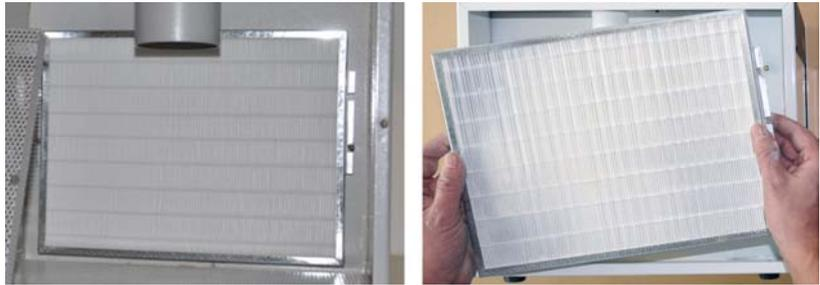
6. Remove the dusty HEPA filter and insert a new HEPA filter.
