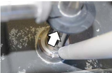
5. Sucking up as much dust as possible from the workpiece axis is recommended. You must also always remove the dust from the bottom of the impact pane of the block axis (see arrow).
