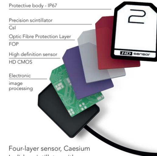
Four-layer sensor, Caesium Iodide scintillator with column-like micro-structures that preserve image quality; intercepts the X-ray beam and converts it into visible light. The Fibre Optics Plate collimates the radiation onto the sensor and protects it against X-ray penetration. The CMOS acquisition device and the electronics convert the light into a high definition digital image.
