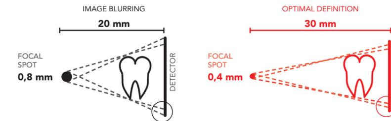
Increased X-ray parallelism and an incorporated collimator allow the RXDC to achieve a source-to-skin gap of 30 cm. The RXDC provides pin-sharp, precise images with outstanding detail.
